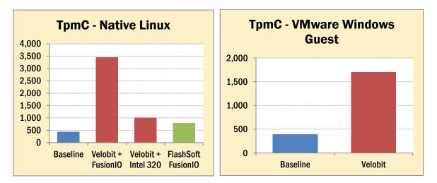
The TpmC score in the native Linux environment with the VeloBit HyperCache read-write SSD cache enabled was approximately *8x higher* than the baseline results. The same test run in the VMware environment with one Windows guest VM was approximately *4.3x higher* than the baseline results in the VMware environment.
