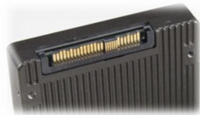
One of the first shipping products to use this SSD-specific form factor was announced in March 2012. This device uses SLC flash, and provides a little less than the 2 GB/s maximum bandwidth supported in the PCIe 2.0 x4 configuration of this product.
