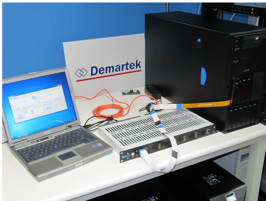
Figure 2 - Torridon 28-drive array controller
