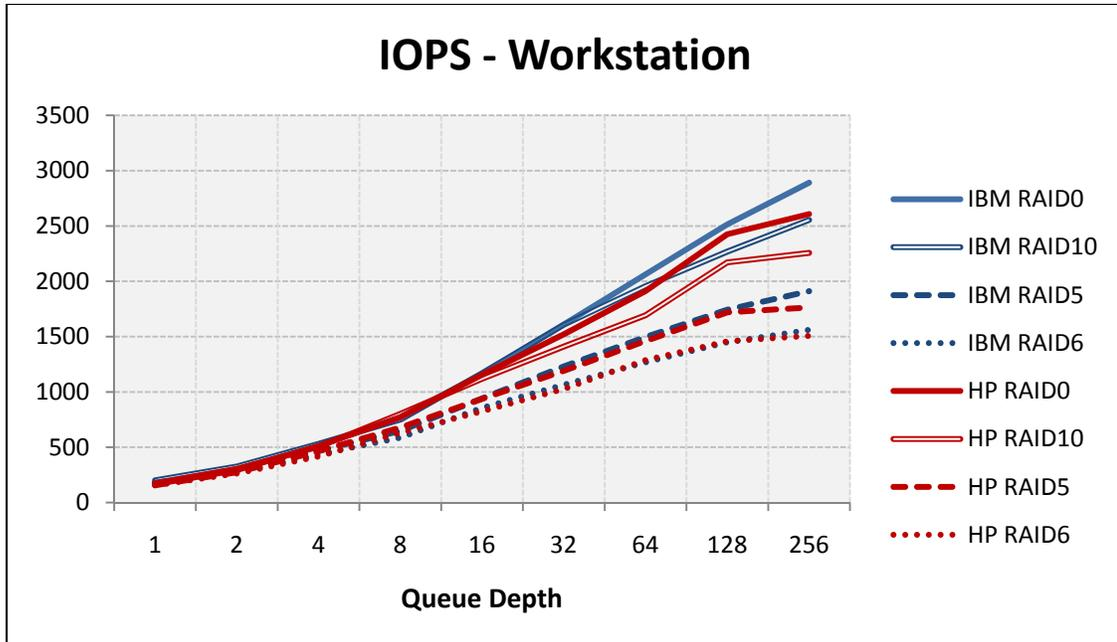
In the operating system drive workload, both controllers appear to scale evenly for RAID0 and RAID10 until the heaviest queue depths, where the IBM controller outperforms the HP controller. For RAID5 and RAID6, the performance is much more even.
