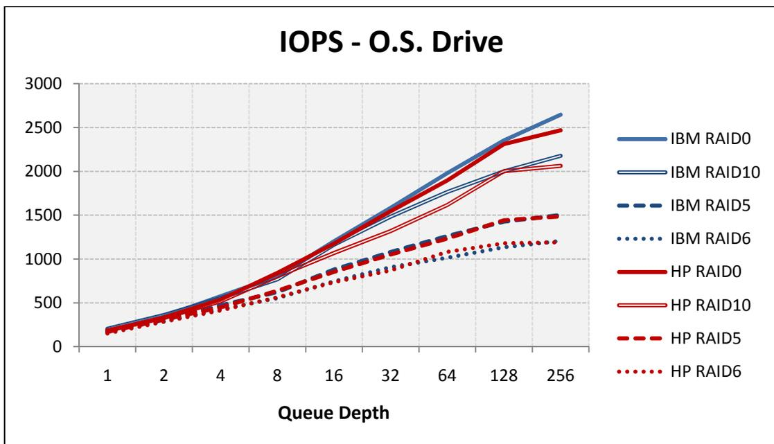
The operating system paging performance is quite different than the other workloads. In this case, the IBM controller has a clear advantage at the lower queue depths, but the HP controller has the advantage in the highest queue depths.
