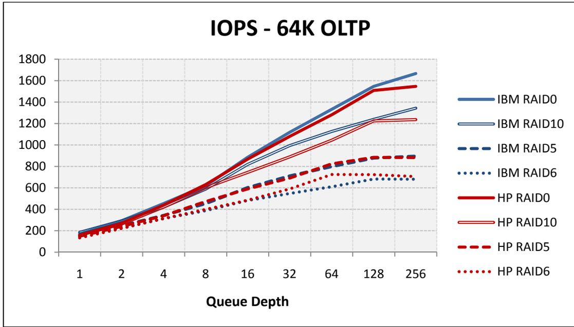
In the email server workload, both controllers appear to scale evenly at the lower queue depths. For RAID0 and RAID10, the HP controller has an interesting peak at queue depth of 128. Note that the HP controller performs better in RAID5 at the heavier queue depths.
