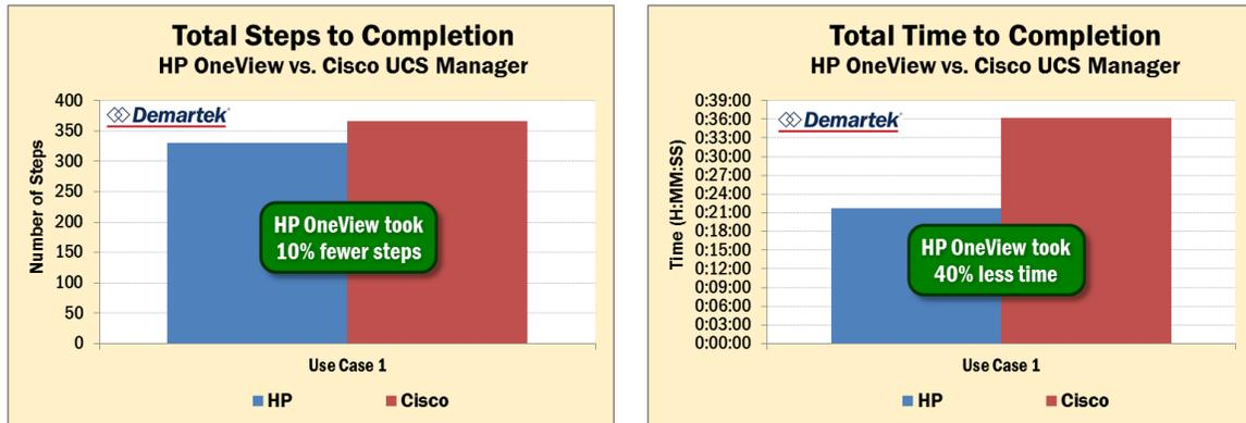
For this use case, we deployed each of the two blade server systems using the respective management software for each system. Each system was reset to factory defaults and deployed. The clock starts when the system is plugged in and/or with any prep work that has to be done before the system is plugged in (such as deploying HP OneView).
