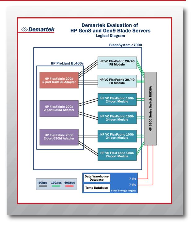
Two different types of VC modules were used in our setup. This impacted our available bandwidth. Each FlexFabric 20Gb adapter has 2 ports of 20Gb. The top adapter, colored red, connects those ports to the 20Gb ports on the HP VC FlexFabric 20/40 F8 module, so it has 20Gb of throughput available on each port. However, the bottom two adapters, colored purple, connect their 20Gb ports to 10Gb ports on the HP VC FlexFabric 10Gb 24
