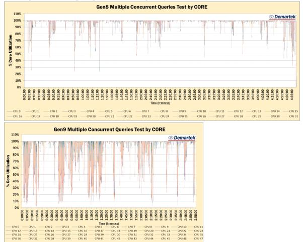
Running 7 queries concurrently ensures that there should be several processor-intensive queries available to take advantage of CPU resources at any point during the test.
