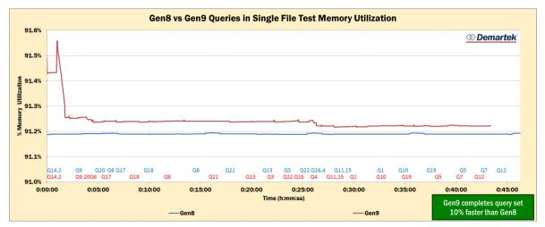
Both systems had 16x32GB DIMMs, giving a total of 512 GB of memory available, and MSSQL Server was capped at 461GB (approximately 90% of available memory on each system). If we look at the scale of the graph, we can see that the memory utilization is mostly due to the 90% allocated to MSSQL server.
