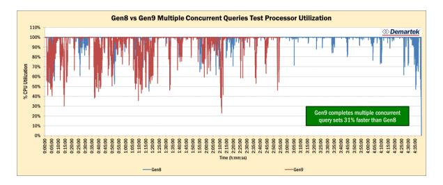
The average processor use over the entire test run was 99.5% for the Gen8 server and 94.6% for the Gen9 server. The Gen9 server still had more processor capability that could be used for other workloads.
