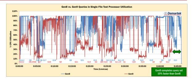
The average processor use over the entire test run was 85% for the Gen8 server and 53.5% for the Gen9 server. The Gen9 server still had plenty of processor capability to spare for other workloads.
