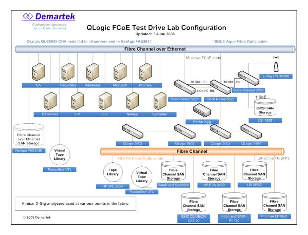
The ten servers listed above were brought by the vendors indicated and were used for testing connections to various devices in the fabric.
