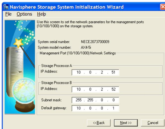
After setting the IP addresses for the AX4 management ports, the IP addresses and other network configuration parameters are needed for the four iSCSI data ports.
