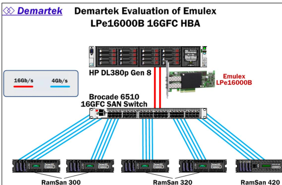
A series of IOMeter tests were run focusing on 100% read, 100% write and 50% read/50% write operations. These tests show traffic flowing in one direction at a time and traffic flowing in both directions simultaneously between the server and storage targets. The IOMeter configuration used was:
