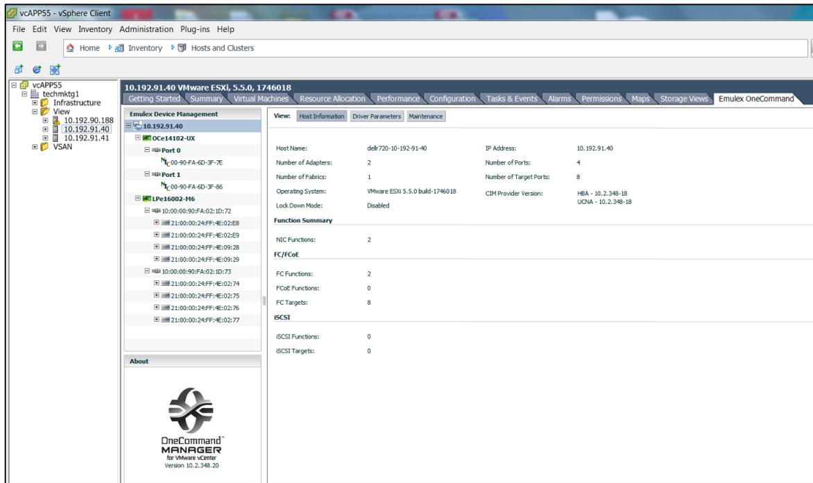
The screenshot shows the vSphere Client interface for host 10.192.91.40. The left pane shows the inventory tree with the host selected. The main pane displays the Emulex Device Management configuration for the host. The configuration shows two ports (Port 0 and Port 1) and an LPe16002-H6 adapter. The right pane displays the host information and a function summary for the adapter.
