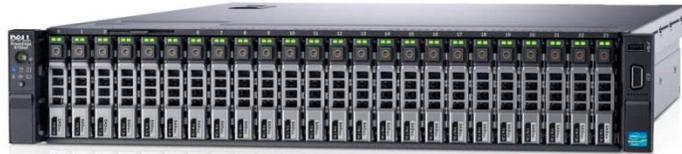
v3 (Haswell) family of processors and provides NVMe support for up to four 2.5" form factor NVMe drives. The server also provides options for external SAS and SATA drive bays in 1.8", 2.5" and 3.5" form factors for maximum flexibility of on-host storage. With up to 768 GB of fast DDR4 RAM and 10 Gb Ethernet available on the motherboard, this server delivers a lot of processing power and I/O potential in two rack units.
