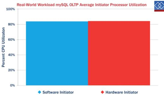
The average processor utilized between the software initiator and hardware initiator did not change much between the two tests.
