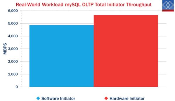
This enabled us to achieve a 20% increase in IOPS and a 16% increase in throughput with the same initiator server processor utilization. We notice again that in the case of a real-world workload, block sizes can vary. The differences in our percent increase for IOPS and throughput shows that average block size changed slightly between the two tests.
