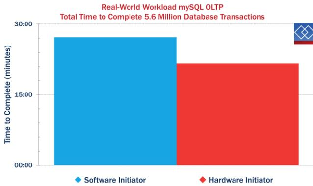
Additional improvements from the offload are a 14% reduction in latency observed at the initiator and a 20% reduction in the time taken to complete 5.6 million database transactions.
