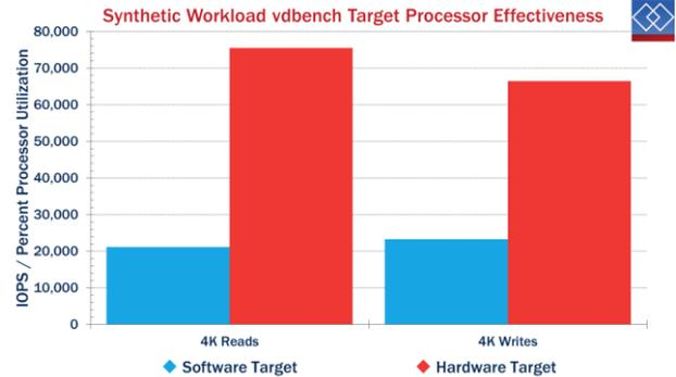
Read IOPS almost tripled with the offloaded iSCSI target, while write IOPS increased by 43%.
