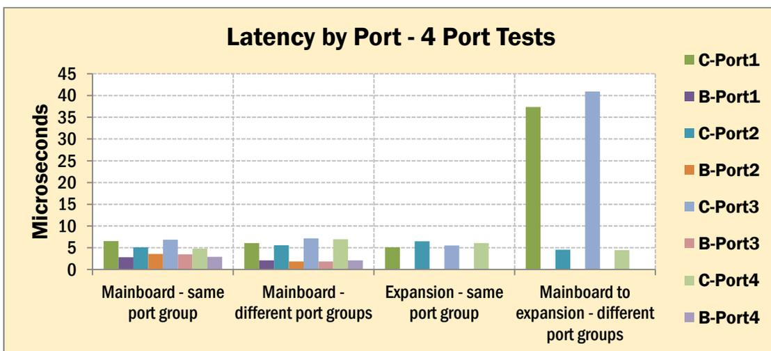
The Brocade switch demonstrated consistently lower latencies for each of the port group combinations, especially when connections crossed port groups.
