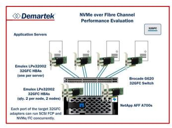
For this test report, Demartek worked with NetApp and Broadcom (Brocade and Emulex divisions) to demonstrate the benefits of NVMe over Fibre Channel on the NetApp AFF A700s, Emulex Gen 6 Fibre Channel Adapters, and Brocade Gen 6 Fibre Channel SAN switches.
