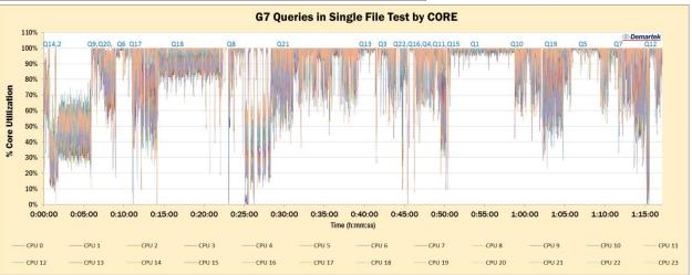
The Gen9 server blade spends less time at full CPU utilization. Queries 18, 1, and 5 push the Gen9 CPU to near 100% utilization just like in the Gen8 and G7, however with multiple cores working in parallel, the completion time for these processor intensive queries is reduced.
