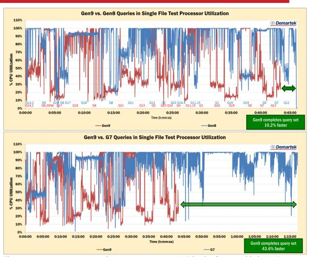
The average processor use over the entire test run was 87% for the G7 server blade, 85% for the Gen8 server blade and 53.5% for the Gen9 server blade. The Gen9 server blade still had plenty of processor capability to spare for other workloads.
