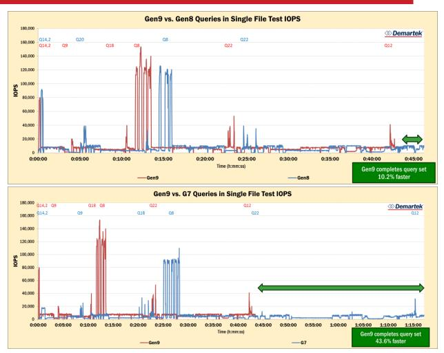
Query 8 stresses the IOPS. Note that the IOPS peaks are highest for the Gen9s and lowest for the G7s, most likely due to each generation having enhanced capability to process the data received as compared to the last.
