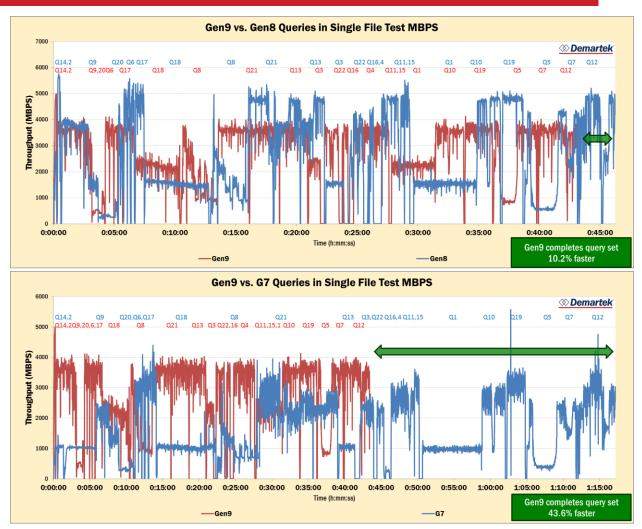
The results show that the Gen9 server blade is able to produce a more steady and predictable load to the storage subsystem, while the Gen8 server blade has many short, high peaks in throughput.
