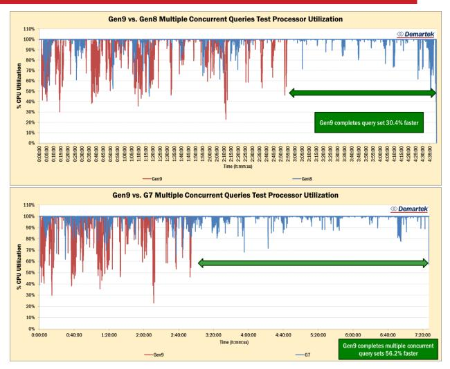
The average processor use over the entire test run was 99.7% for the G7 server Blade, 99.5% for the Gen8 server Blade and 94.6% for the Gen9 server Blade. The Gen9 server blade still had more processor capability that could be used for other workloads.
