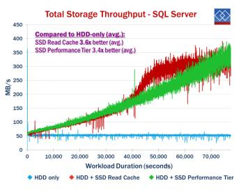
These performance improvements obviously came with corresponding increases in throughput and IOPS as demonstrated in Figure 2. We saw throughput increase by a factor of 3.6 with read caching and 3.4 with SSD tiering, from a baseline of approximately 50 MB/s.
