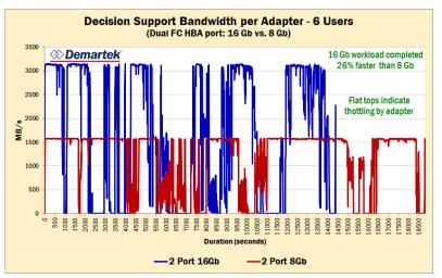
When running this test with the HP StoreFabric SN1000E 16Gb FC HBA, the time to complete the run was 26% faster than the time required by the 8Gb adapter. This reduced the time to complete the workload by approximately one hour.
