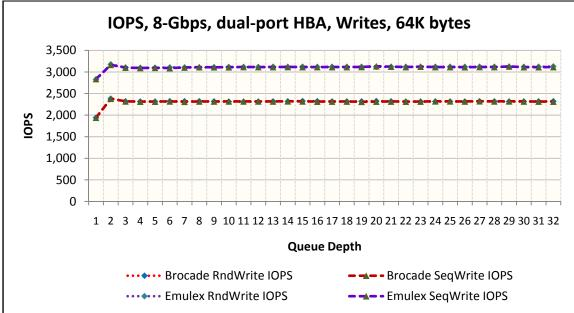
For write performance, the Emulex HBA was noticeably faster than the Brocade HBA for all block sizes and queue depths up through 64K block size. Above 64K block size, the HBA write performance of the two brands was nearly identical.
