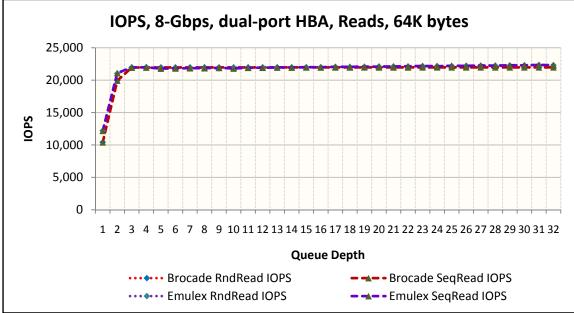
In many cases, the read performance for both HBAs was very close. At the smaller block sizes, they were nearly identical. At the mid-range block sizes, the Brocade HBA was slightly faster, depending on queue depth. For the larger block sizes (128K and greater) the Emulex HBA was noticeably faster.
