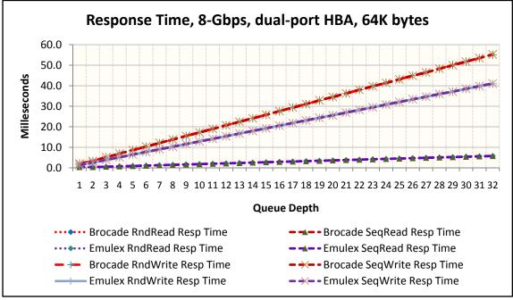
The response time of the Emulex HBA was generally less (better) than the Brocade HBA, especially for writes. The read response times were very close, with the Emulex HBA generally having a slightly better response time. Response time is a measure of the time it takes to get a response from an I/O request.
