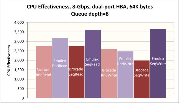
The CPU effectiveness, a measure of CPU utilization for the work performed, was generally better for the Emulex HBA.
