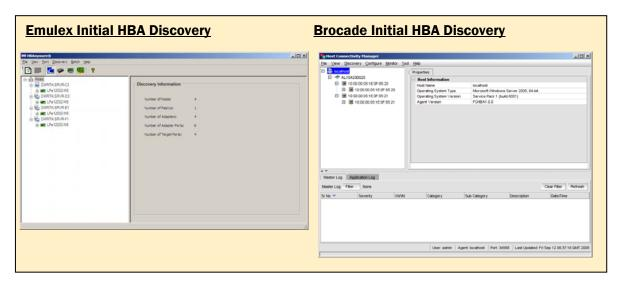
Emulex HBAnyware provides a Host View and a Fabric View, showing all Emulex HBAs visible in the SAN fabric. The Fabric View shows the host name associated with each HBA. A single click can switch between Host View and Fabric View as shown below.
