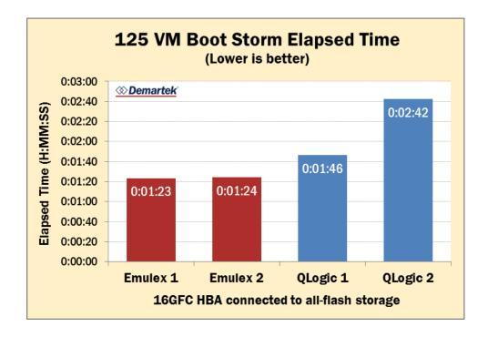
The elapsed times to complete the boot sequence for all 125 VMs were significantly faster and more consistent with the Emulex LPe16002B FC HBA, leading to a higher degree of confidence and predictability for the VDI boot procedure. By contrast, the QLogic QLE2672 FC HBA displayed higher variability and slower performance, in one case taking almost twice the amount of time to complete the full set of virtual machines.
