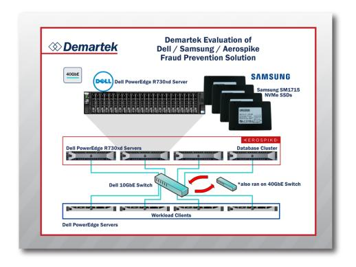
Four cluster servers were chosen for this testing strictly for ease of deployment. Aerospike easily scales to support larger datasets by simply adding additional cluster nodes. A reasonable comparison to larger environments can be made by multiplying the performance results to the scale factor of larger clusters.
