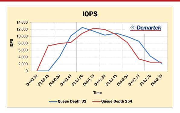
Most of the performance increase may be attributed to the VM Queue populating slightly faster, with the time taken to put all VMs into the queue reducing by 24%. We can see the results of this in the graph below where there are more VMs in queue at the beginning of the test, which gives the queue depth 254 configuration a head start.
