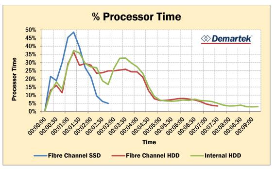
HDDs can improve performance by using caching and increasing queue-depth, but do not compete with solid state drive performance.
