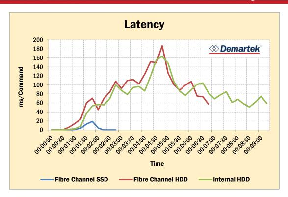
In addition, solid state drives had the throughput necessary to efficiently handle storage requests from the starting VMs.
