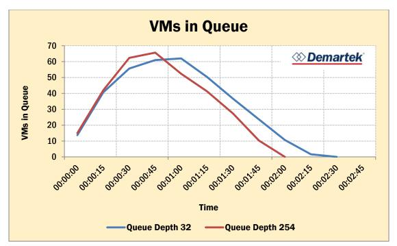
A graph of VMs completing boot shows again how the queue depth 254 configuration gets a head start. The time before the first VM completes boot is shorter when the queue depth is increased to 254, but the slope of both lines for queue depth 254 and queue depth 32 are the same once the boots are started, suggesting that the advantage was again that the first boots were completed faster, giving a head start when the queue depth was increased.
