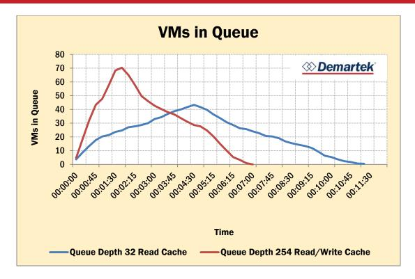
The rate at which VMs were able to complete boot was faster for queue depth 254 than it was for queue depth 32, as evidenced by the slope of these lines. Again this shows that the bottleneck was mostly due to the HBA settings.
