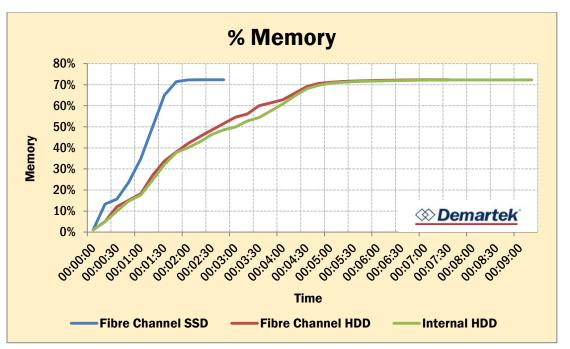
SSDs dramatically outperformed the HDDs in a bootstorm, regardless of configuration. This appears to be due to their low latency. Latency for HDDs increased as more VMs were added to the queue, but latency for solid state drives stayed low the entire time. As the ESXi libraries waited for responses from storage, lower latency SSDs were able to increase ESXi library availability, enabling more VMs to start their boot sequences.
