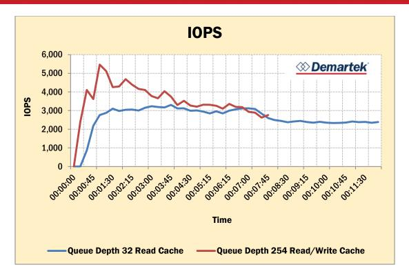
As mentioned previously, ESXi shared libraries wait for a response from storage while powering on VMs, requiring software power-on requests to be delayed to avoid ESXi errors. Below we can see that the reduced latency with queue depth 254 enabled the VM queue to be populated 64% faster, which enabled more VMs to boot at the same time and all VMs to boot faster.
