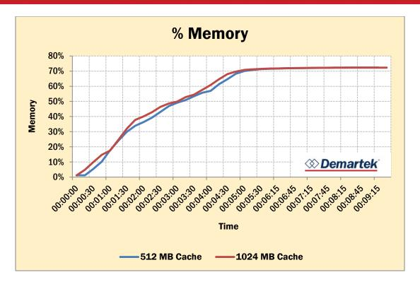
However, we found that bootstorms are a cache-friendly workload. Increasing cache size to 1024MB enabled the ESXi software to handle VM start requests faster, which lowered the number of VMs in queue and caused the queue to be completed faster. Boot times were reduced for all VMs by an average of 18%.
